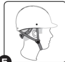
To remove the helmet, release the chin strap by pressing together the tips of the male side of the snap buckle (Fig. 6).
